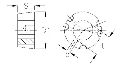
$\begin{array}{lll} b & = 20 \\ Bore & = 75 \\ Bush type & = 3525 \\ D1 & = 127 \\ S & = 64,9 \\ Screw size & = 1/2 \times 1 \ 1/2" \\ t & = 79.9 \end{array}$
